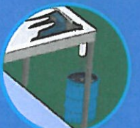
Flat roof without adequate drainage
